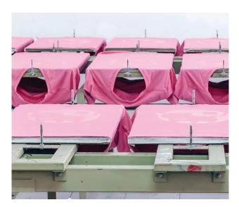
**Screen Printing:** The process of printing images on a t-shirt or other substrate using screen, mesh and ink. The image is transferred by the pushing or pulling of a squeegee.
