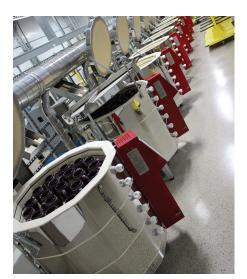
BELOW Fired and glazed mugs are moved into a shipping area for packing. LEFT Products are loaded into computer-controlled kilns with built-in sensing and safety features, which are controlled internally and via the internet.
