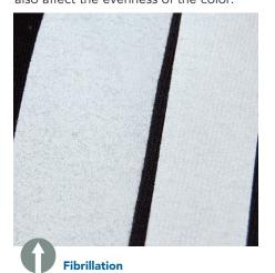
Fibrillation can occur in screen printing and direct-to-garment printing. Using a heat press to flatten your garment before direct-to-garment printing can help smooth out the fibers. Printing a good underbase will help smooth the fibers for screen printing as well.
